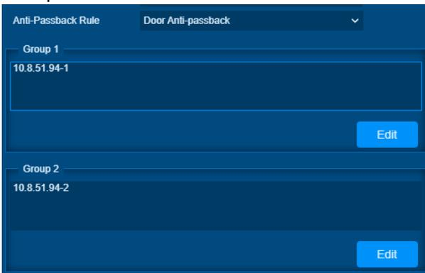
Personnel can only enter Door A (IN) and exit from Door B (OUT), if Enter Door A (IN) and exit from Door A (Out), Device will deny access and send event 'Anti-Passback'
