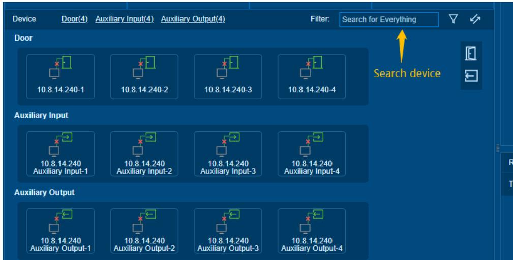
**Filter device:** System support filter devices by door status, relay status, auxiliary input status and auxiliary output status.
