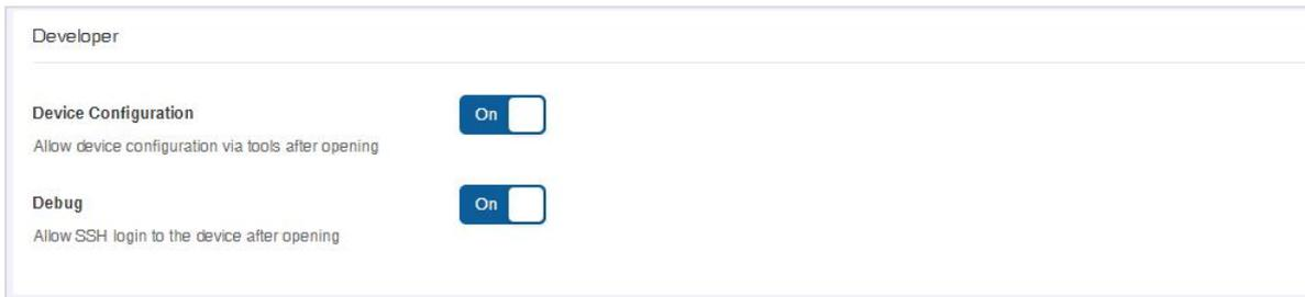
**Device Configuration:** factory device default on (turned on to allow demo tool to set device parameters).
