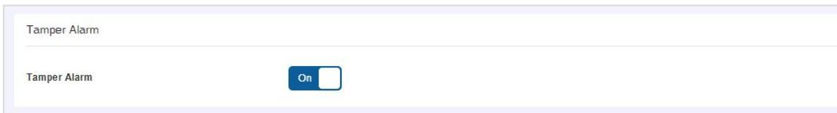
**Tamper Alarm:** factory device default on (when turned off, the device does not detect the tamper function).
